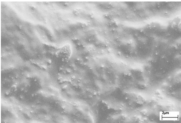
Fig. 7 SEM photograph of impact fracture surface of SI system ( \phi_f = 3\% )
